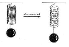
extension of spring = 0.6 - 0.5 = 0.1 m  $E_e = \frac{1}{2} \times 800 \times 0.1^2$ Stored elastic potential energy of the spring = 4 J
