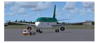
When a pushback truck is used to move an aircraft, it does work.
