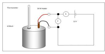
**Example:** When the heater was left on for 5 mins, the heater supplied 10 800 J of thermal energy to the aluminium block.
