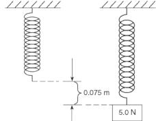
The amount of stored elastic energy  $(E_e)$  can be calculated using the following equation:
