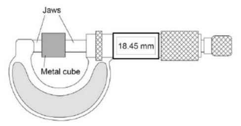
(a) The resolution of the micrometer is 0.01 mm
